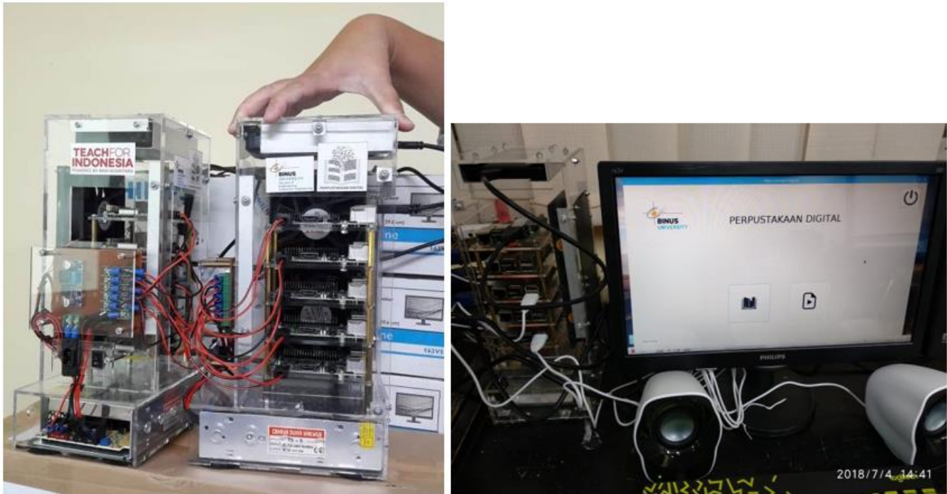
Figure 1. (Left) Raspberry Pi's cabinets, which consisted of 5 minicomputers per cabinet. (Right) the system was fully set up.
